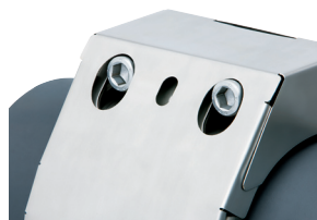
Step 3 Ensure that the screw heads remain accessible
