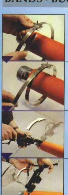
R-LOC CLAMPING SYSTEMS: INSTRUCTIONS FOR USAGE (Bands & Buckles or Ties)
